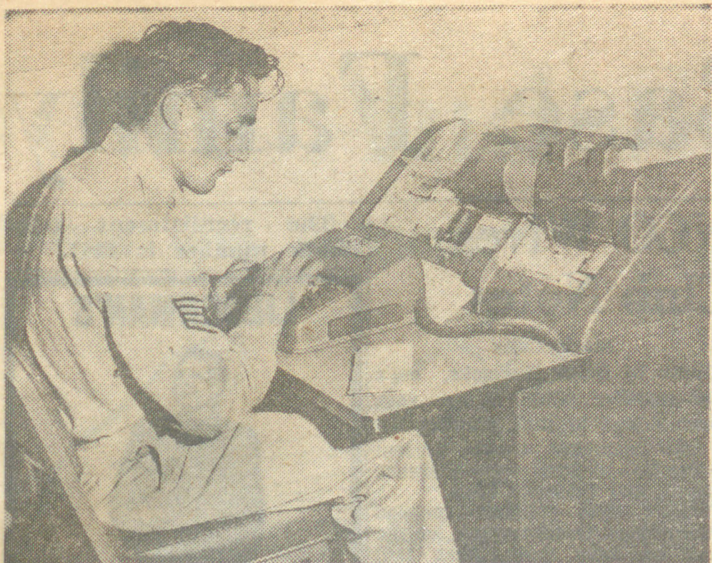
NEW MACHINES —Dow's Personnel section received their first IBM machines recently. Here, SSgt. J. Roger D. Theriault, NCOIC of the Machine Shop, is seen using the printing card punch machine. This new machine saves time, money and is more efficient for posting of records.
