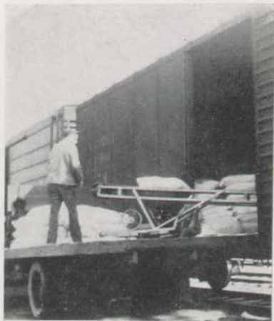
The power conveyor shown moving bagged salt has cut in half the time used in loading and unloading freight other than bulk at Eastport. The conveyor, put in use by E. B. Scott, contract trucker for the Maine Central at Eastport, can handle 600 bags of salt per hour. The equipment results in quicker release of cars and better service to shippers.
